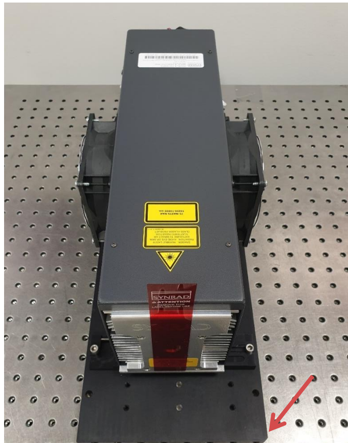
Figure 8: Laser fixed on the mounting rail with four 1/4-20 UNC cap screws (the position of the notch is highlighted)
