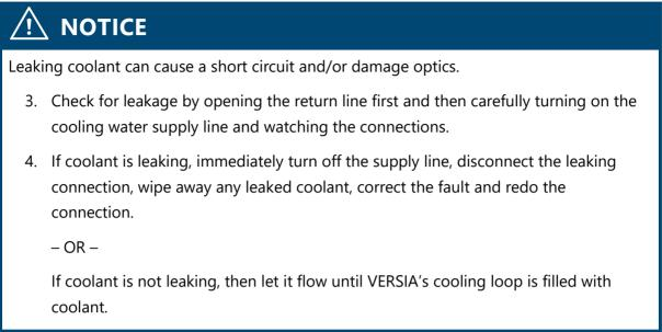
5. Turn off the coolant supply line first and then the return line.
