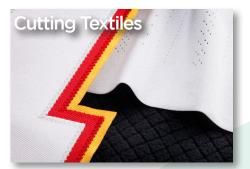
When cutting many natural and synthetic textiles cut edge charring or melting is caused by excessive heat build-up in the material. High peak power and fast pulse rise time eliminates this issue, expanding the range of materials for laser processing.
