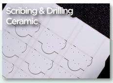
The high peak power is essential to minimizing heat build-up and avoid cracking when processing brittle materials such as alumina, ceramic and quartz glass. Excellent beam quality allows for very small features and clean symmetric holes.
