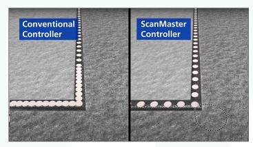
Skywriting – delivers uniform laser density when processing complex shapes and tight corners to avoid "burn marks" caused by over-processing.
