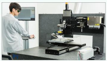
**SyncMaster** – advanced laser scanning head and XY linear stage synchronization expands work field size and fits production environments with unmatched accuracy and speed.
