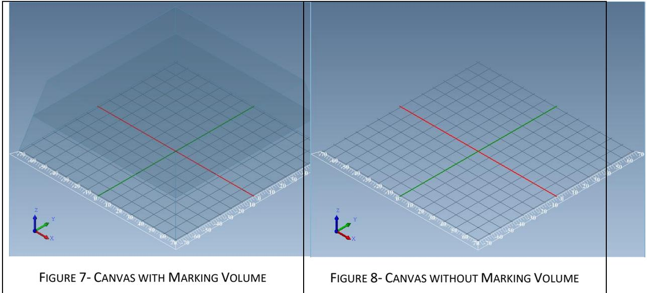
Any 3D models or sections of 3D models which are placed beyond the marking volume will not be marked by the scan head.
