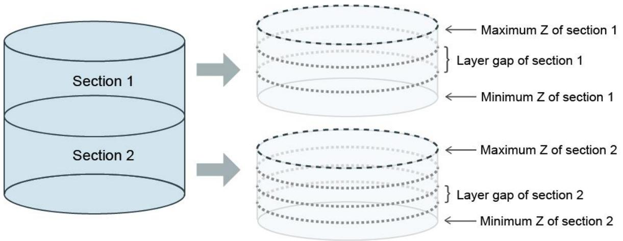
FIGURE 17- SECTIONS AND LAYERS OF ENGRAVING
