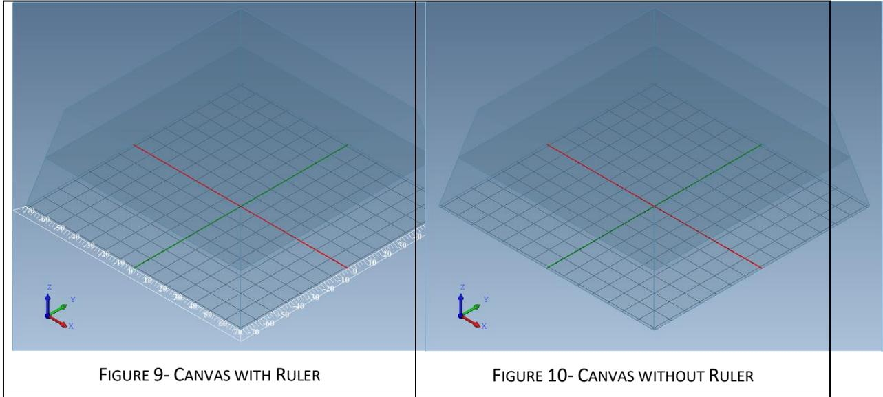
A ruler is displayed along the **X** and **Y** axis of the drawing canvas in order to help you adjust the position of the 3D model in the drawing canvas.
