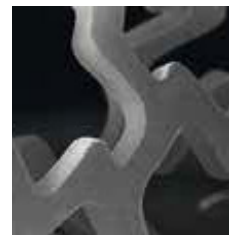
Cutting of coronary stents 100 \mu\text{m}
