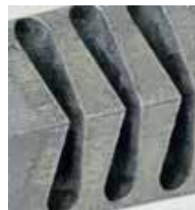
Microprocessing of co-balt-based carbide 200 \mu\text{m}
