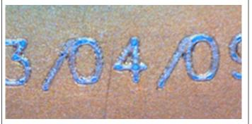
10.2 µm: Clean, consistent, and highly visible mark.
