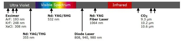
$CO_2$  lasers have long wavelengths, around 9.3 – 10.6  $\mu$ m, with 10.6  $\mu$ m as the most common. These wavelengths pair nicely with the absorption spectrum from polymers, ceramics, textiles, natural materials like paper or wood, and certain metals. By contrast, the shorter wavelength YAG or Fiber lasers tend to have better absorption in metals.
