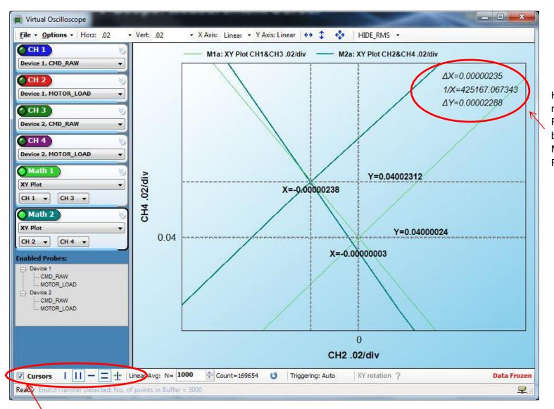
Here displays measurement result. For this case, unit for both CMD\_RAW and MOTOR\_LOAD is Radians.
