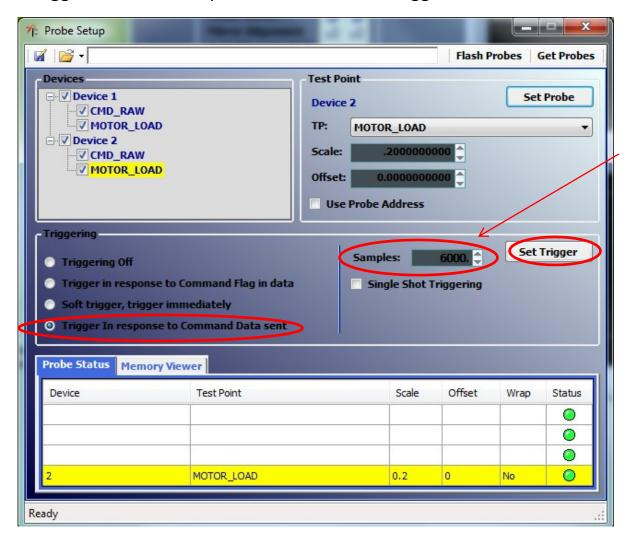
If sample size is too small, virtual scope will not see complete pattern. If sample size is too high, virtual scope will see multiple passes/traces
