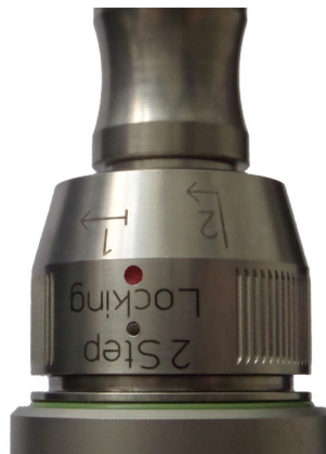
Figure 7.1.: QBH fiber coupling with plugged in fiber
