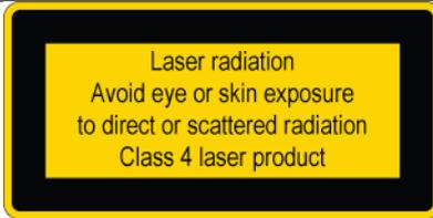
Find the Class 4 laser product label at the right scan head side in beam direction.
