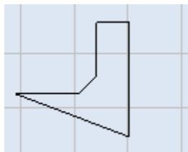
FIGURE 509: THE FINISHED CHAMFER
