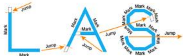
Laser On Delay Too Long: marking starts too late, skips points
