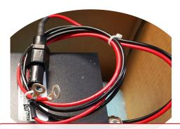
**4.3.** Drape the wire harness across the top of the laser housing when lifting.
