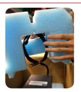
4.2. Push the wire harness through the notch in the foam.
