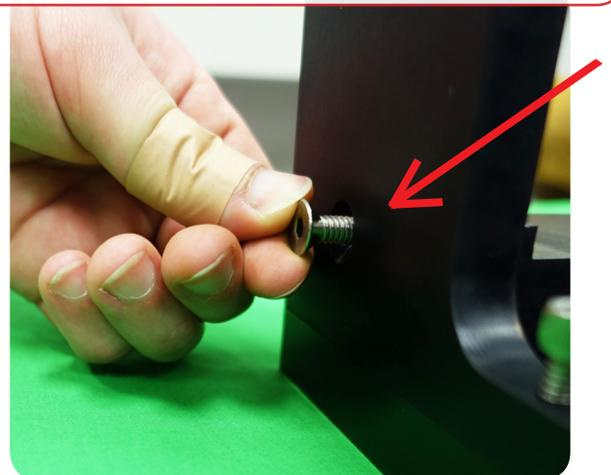
7. Assembling the **front** end of the rail, **make sure the notch is not at the front end of the laser. See the figure(s) above before going on to the next step.**
