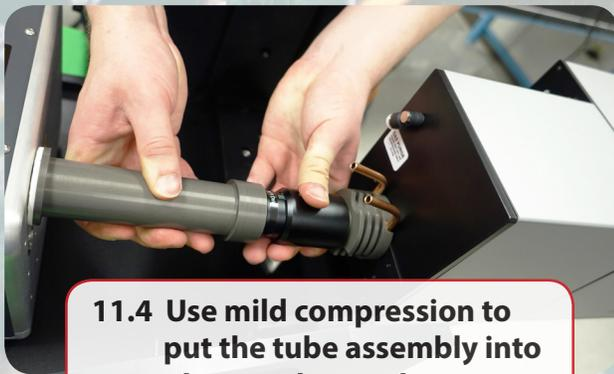
**11.4 Use mild compression to put the tube assembly into place as shown above.**
