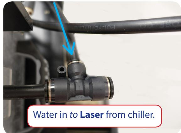
**Note:** Assure the port for water out from Marking Head is connected to the water out from Laser to chiller. Same is true for the water in from the chiller to the Marking Head/Laser.
