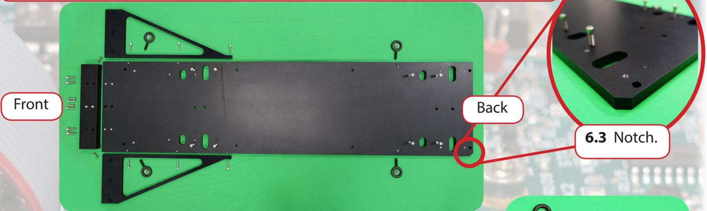
**6.1** Install the long laser bolts after the laser is mounted to the rail.
