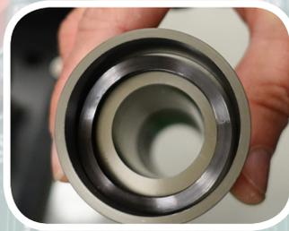
**11.2 Place the wavy gasket into the assembly as shown above.**
