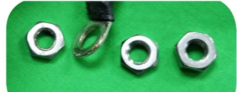
16.1 Nut order on attaching the power cable.
