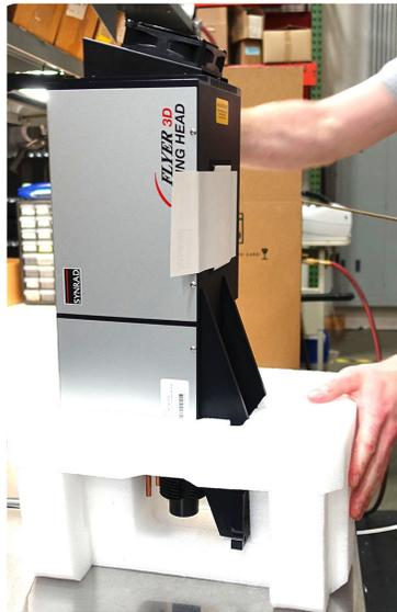
3.1 Remove and retain the marking head foam.
