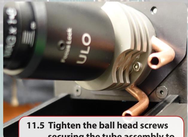
**11.5 Tighten the ball head screws securing the tube assembly to the Marking Head.**
