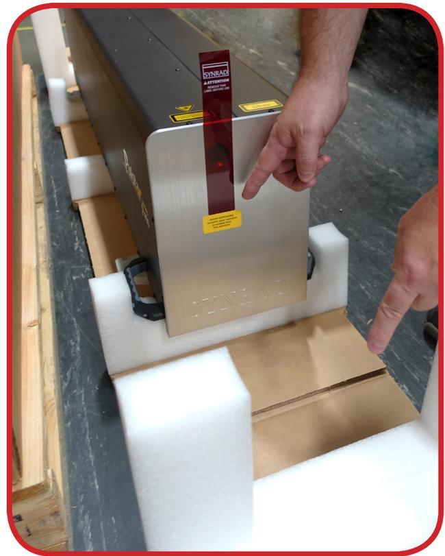
**4.6** Notch-less foam end is for the front end of the laser.
