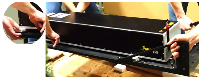
4.6 The loop/rail sidebars can also be used to unseat the laser from the foam before lifting it out of the crate.
