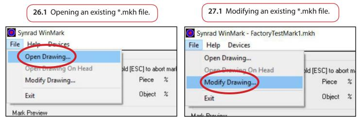
**27.** To add an Admin password so operators cannot modify a drawing select '**Modify Drawing...**' which then opens the WInMarkpro application.
