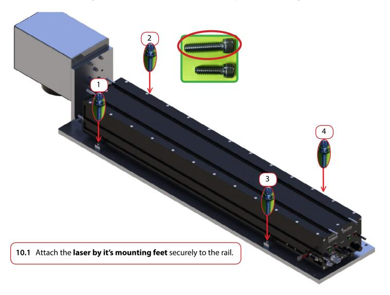
Important Calibration void if shim bolts are adjusted, if your laser has mounting feet as shown above, careful not to carry or handle the laser by the feet to minimize misalignment risk.
