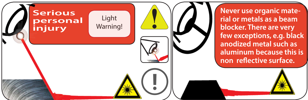
Figure 2-2 Always wear safety glasses or protective goggles with side shields to reduce the risk of damage to the eyes when operating the laser.
