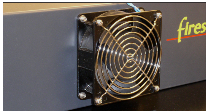
Maintaining the recommended operating temperatures for sealed CO 2 lasers is critical. The use of secondary cooling mechanisms like fans or flowing water systems are commonly added to assist cooling.
