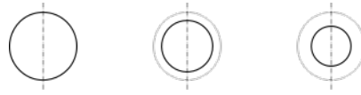
Figure 5.7: Partially compensated output (with frequency rising from left to right); compensation of radius still due
