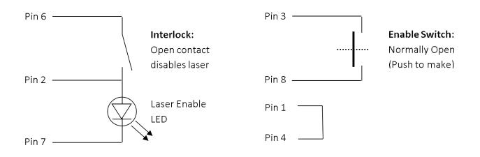
If the Interlock connection is broken or if the laser head or controller overheats, the laser will shut down. The Interlock connection must be re-made or the temperature restored to normal before the laser can be re-started.
