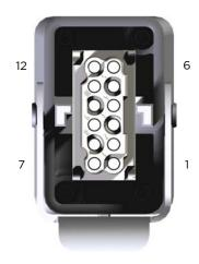
Connector type of the "safety" connector: 12 pin socket HARTING HAN DD module 09 14 012 3101 with housing 09 14 001 0301
