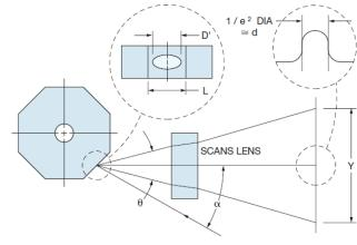
FIGURE 2: SCAN SYSTEM WITH SCAN LENS
