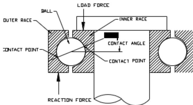
Each bearing type has a unique rating for its load carrying capacity. The load capacity is a function of the bearing geometry at the ball/raceway contact points (number of balls in the bearing, the size of the balls, the contact angle of the balls to the raceway, etc.). If a load that exceeds the rated capacity is applied across the bearing, the raceways and/or balls will permanently deform. This deformation is called brinelling.
