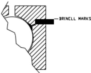
Brinelling a scanner's bearings results in unwanted displacement of the polygon, reduced speed stability, audible noise, and repeatable vibrations.
