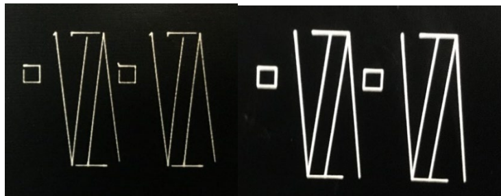
Figure 9: Example of badly adjusted delay settings (left) and well-adjusted delay settings (right)
