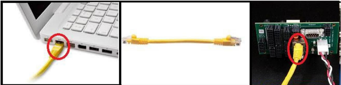
**Figure 2 - EC1000 - Connect an Ethernet Cable from PC to the EC1000 I/O Module**
