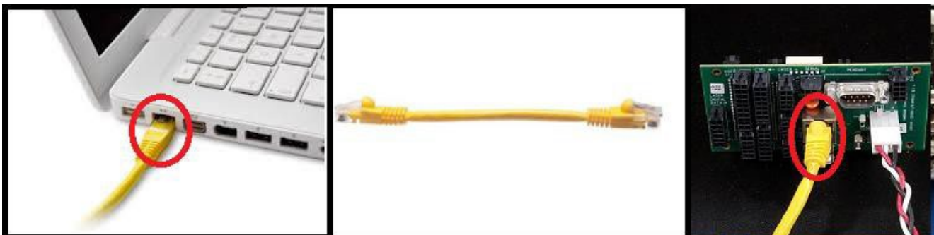
Figure 3 - EC1000 - Connect an Ethernet Cable from PC to the EC1000 I/O Module
