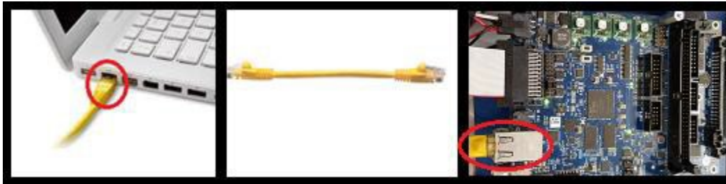
Figure 1 - SMC- Connect an Ethernet cable from PC to the Controller
