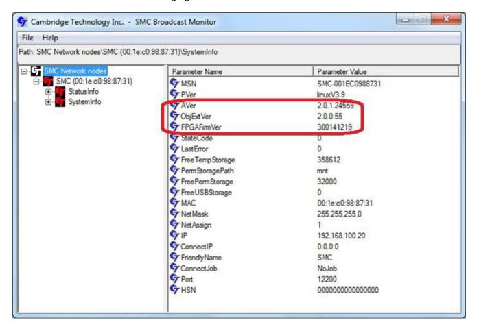
Figure 5 - SMC Broadcast Monitor shows SystemInfo
