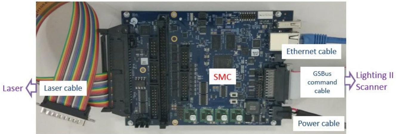
Figure 4 - The SMC with the GSBUS interface to a Lightning II scanning system
