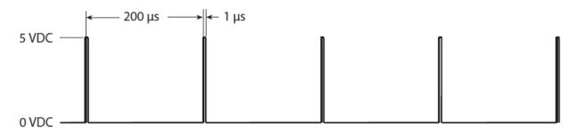
Figure 4-3 Tickle pulse waveform.
