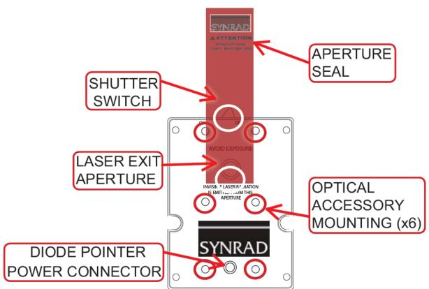
Figure 3-1 48-1/48-2 Front panel controls and indicators.
