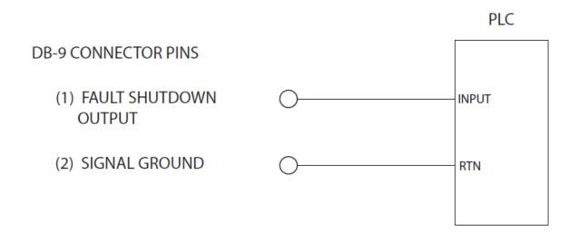
Figure 4-13 Fault Shutdown Output to PLC input.
