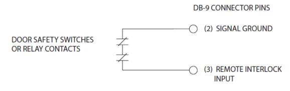
Figure 4-10 Remote Interlock circuit.
