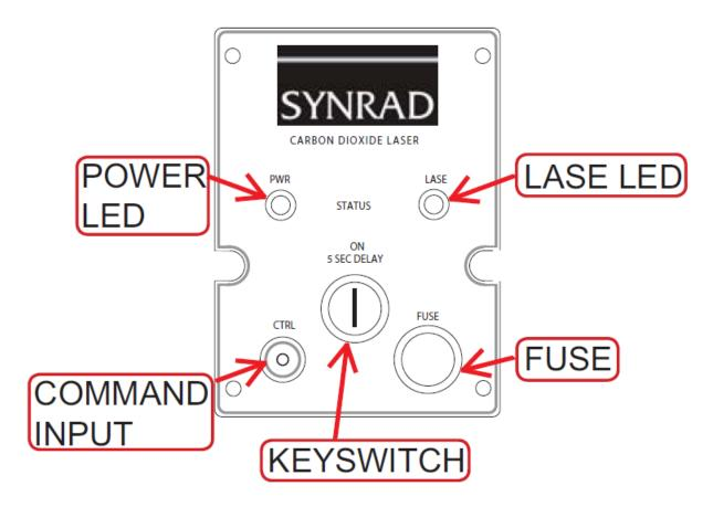
Figure 3-2 48-1/48-2 Rear panel controls and indicators.
