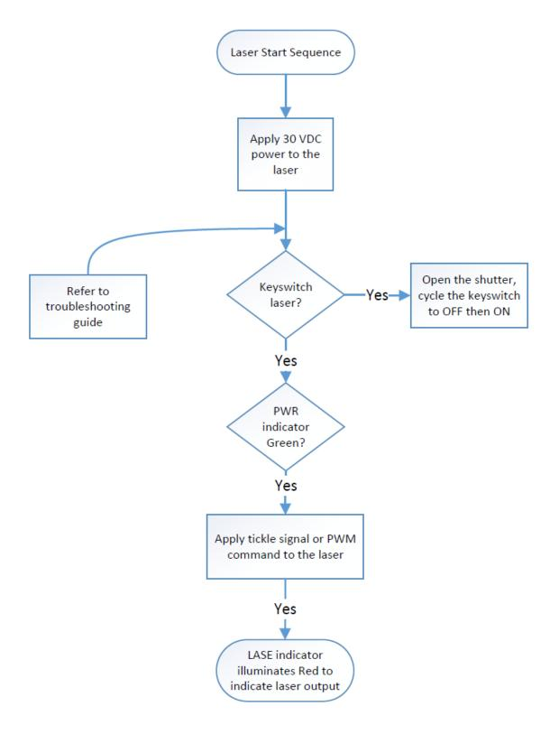
Figure 5-1 48 series operational flowchart.
