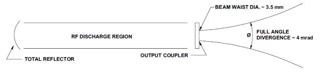
Figure 4-1 beam characteristics
