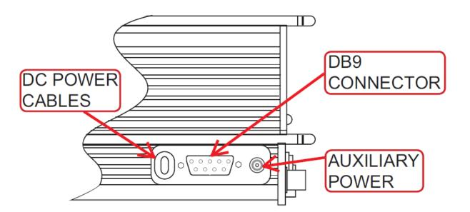
Figure 3-3 Side panel controls and indicators.
