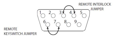
Figure 4-7 Factory-installed DB-9 jumper plug wiring.
