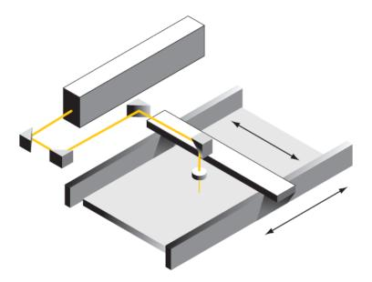
Figure 4-2 "Flying optics" beam path
