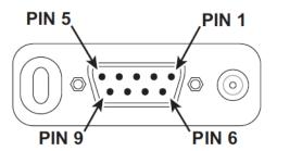
Figure 4-8 Physical layout of Series 48 DB-9 Connector.
