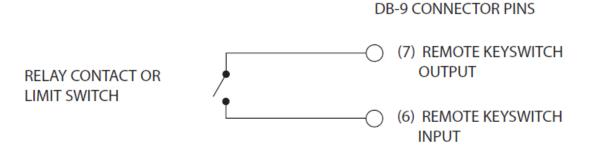
Figure 4-9 Remote Keyswitch circuit.
