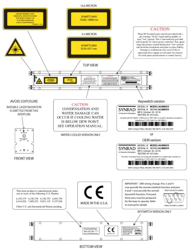
Figure 2-1 Hazard label locations (48-1 example).
