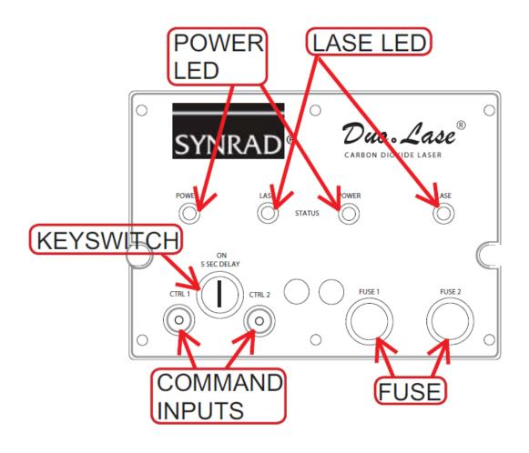
Figure 3-5 48-5 Back panel controls and indicators.
